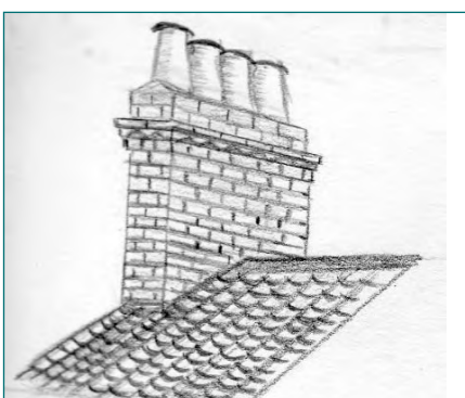
Projecting chimney 'drip'
